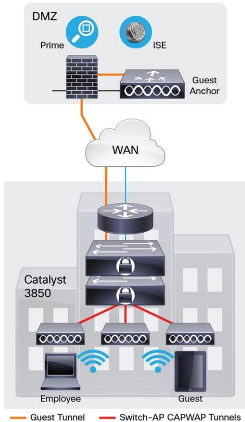
The new 12-port and 24-port SFP+ or SFP-based Cisco Catalyst 3850 models as well as the nonstackable 48-port SFP+ model can also be used in the branch to aggregate traffic from smaller access switches through fiber links for more secure and EMI-sensitive deployments (Figure 11).
